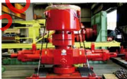
BOP BLOW OUT PREVENTER
